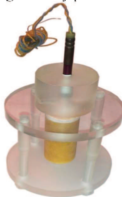
Fig.2. Assembly with TNT/RDX charge of 40 mm in diameter.
