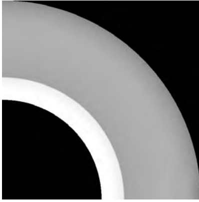
Fig. 4. Electrostriction flow between cylindrical electrodes (black). High-density phase is shown in white. Initial state of a liquid was \tilde{\rho}_0 = 1.8 , \tilde{T} = 0.9 , t = 173 (in units of Fig. 3). Grid size 600 \times 600 . h = R/300 .
