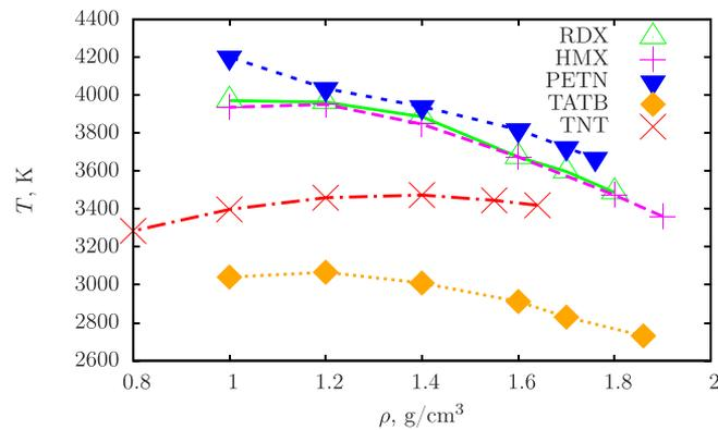
FIG. 2. Temperature at the CJ point, based on data from work.<sup>15</sup>
