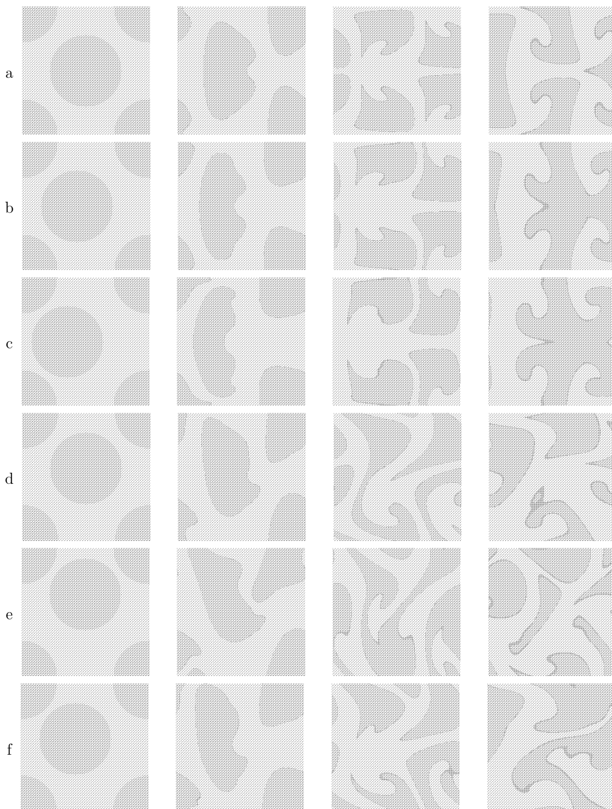
Figure 3.8. Flow for the "diagonal" drop layout. Displacement of the central cylinder is a : (\Delta x, \Delta y) = (0, 0) , b : (\Delta x, \Delta y) = (-d/8, 0) , c : (\Delta x, \Delta y) = (-d/4, 0) , d : (\Delta x, \Delta y) = (0, d/8) , e : (\Delta x, \Delta y) = (0, d/4) , f : (\Delta x, \Delta y) = (-d/8, d/8)
